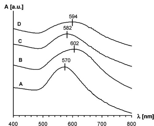
**Figure 7.** UV–vis spectra of a single sample of  $\text{SiO}_2\cdot\text{Au}$  clusters after successive reaction with octadecanethiol (A, C) and butanethiol (B, D). All spectra were corrected for turbidity by subtracting the spectrum of pure  $\text{SiO}_2$  particles in methanol.
