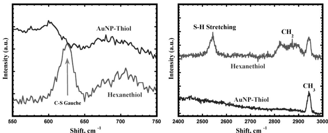
**Figure 6.** Comparison of SERS spectra for the  $\text{SiO}_2\cdot\text{Au}-\text{SC}_6\text{H}_{13}$  composite and for pure hexanethiol. The weakness of the C–H bands in the spectra is due to the reduced detection sensitivity of the analytical setup at 1.00 mm, which is five times weaker than at 800 nm.
