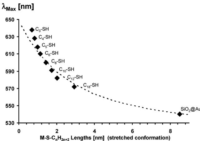
**Figure 5.** Experimentally observed positions of the UV-vis absorbance maxima plotted versus the lengths of the thiols (diamonds) and theoretical fit (see main text, broken line).
