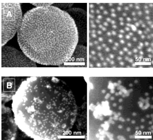
**Figure 2.** Morphology of the gold–silica core–shell-type composite as observed by the SEM: (a) as-synthesized, and (b) after 10 min of treatment with an aqueous solution of 0.01 M of potassium bromide.
