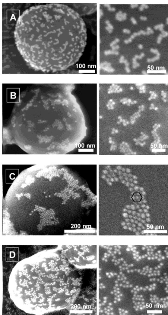
**Figure 3.** Scanning electron micrographs of SiO<sub>2</sub>·Au nanoparticle clusters after reaction with alkanethiols of variable alkane group lengths: (A) propanethiol, (B) hexanethiol, (C) dodecanethiol, and (D) octadecanethiol. Magnified regions of the corresponding clusters are shown on the right.
