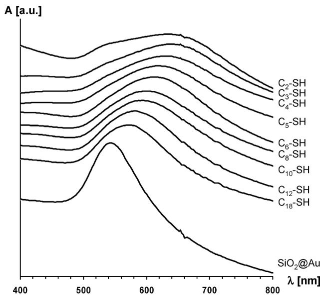
**Figure 4.** Electronic spectra of  $\text{SiO}_2 \cdot \text{Au}$  clusters before (bottom) and after reaction with alkanethiols  $\text{C}_n\text{H}_{2n+1}\text{SH}$  ( $n = 2, 3, 4, 5, 6, 8, 10, 12, 18$ ). All spectra were corrected for turbidity by subtracting the spectrum of pure  $\text{SiO}_2$  particles in methanol.
