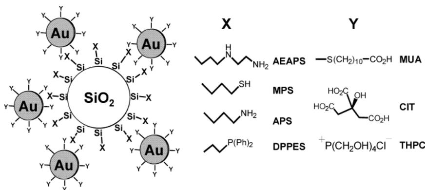
**Figure 1.** Schematic composition of electrostatically and covalently bonded silica-gold core-shell-type nanoparticle composites.
