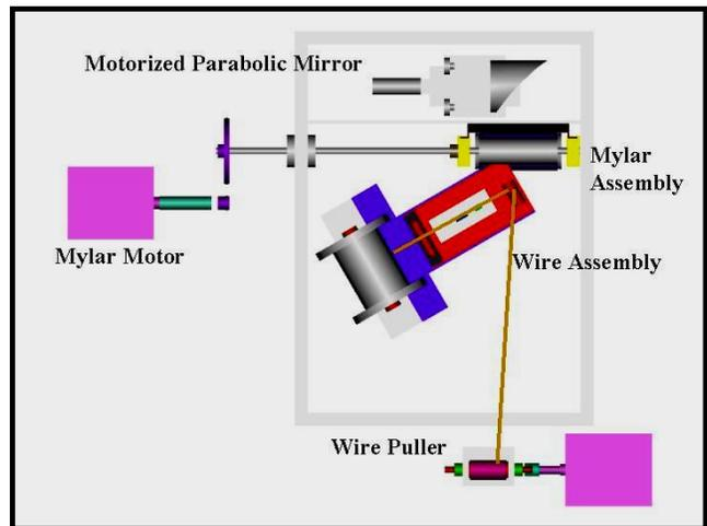
Figure 2. Target apparatus in the LEXS.
