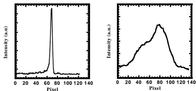
Figure 4. Spot size measurements of broad and sharp diffraction patterns. The size of the pixel is 22  $\mu\text{m}$ .
