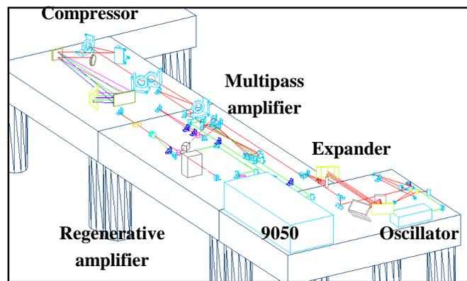
Figure 1. Schematic of UC Davis terawatt laser system.
