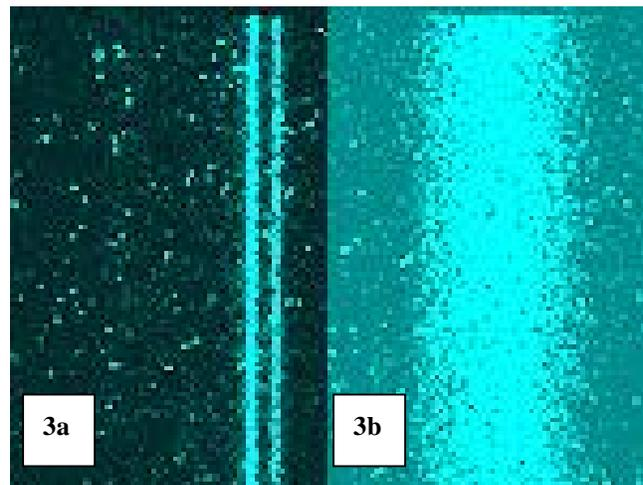
Figure 3. Sharp (3a) and broad (3b) diffraction patterns from the same target (Cu) under different focusing conditions. The left panel (3a) is obtained with a sharp focus and has a much high flux than that of the right, which is emitted from a much larger spot.
